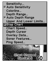
Sonar Menu with Stop Chart command selected. The box is unchecked, indicating that the chart is scrolling across the screen.
